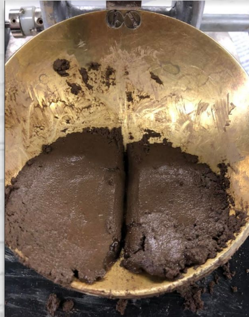
Photo 7: Liquid Limit Testing (Casagrande Cup)
